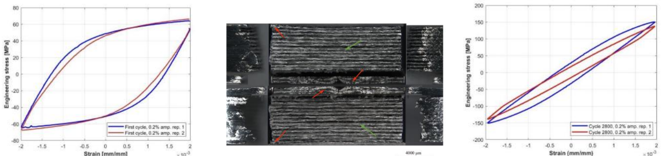
Figure 1. Representative cyclic stress–strain hysteresis loops obtained from adhesively bonded laminated thin aluminium sheet specimens tested at a total strain amplitude of 0.2%, together with corresponding fracture surface features showing fatigue crack growth patterns.
