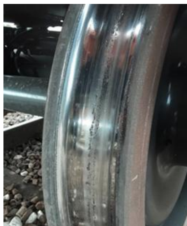
Figure 1 – Severe Rolling Contact Fatigue damage on the wheel tread induced by the combination of thermal loads and mechanical loads.
