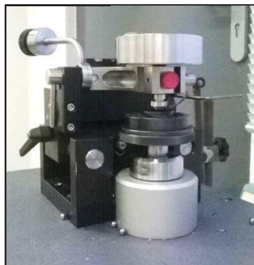
Figure 1 - Tribological test on a stainless-steel specimen coated with Al_2O_3 .
