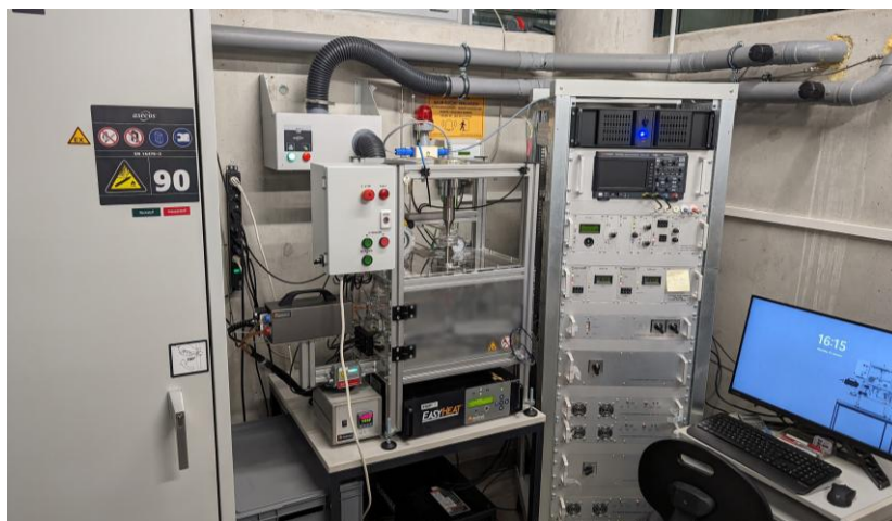
Figure 1 - Testing facility for VHCF test in hot hydrogen gas at elevated pressures at BOKU Vienna.
