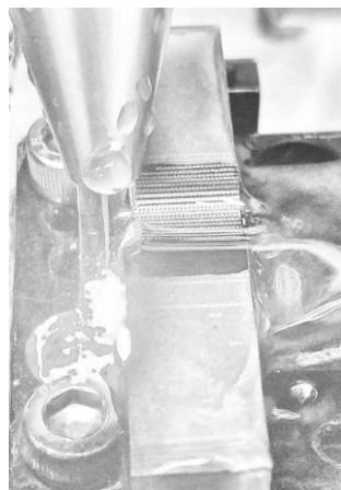
Figure 1 – Coaxial Laser Shock Processing accurately implemented on turbine blade coupons
